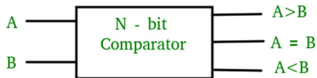
Figure 2: N - bit Comparator
